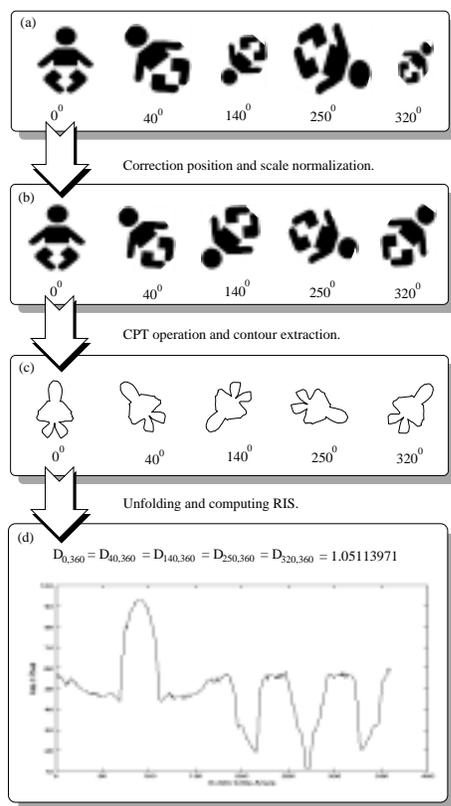
**Figure 2. Diagram of RIS approach to extract rotation invariant feature.**
