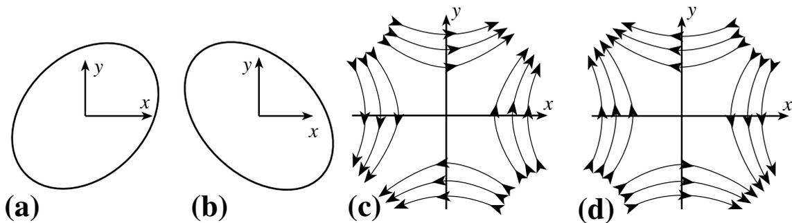
**Fig. 26.2:** Physical manifestations, in a particle’s local Lorentz frame, of  $h_{\times}$  gravitational waves. (a) Deformation of an initially circular sphere of test particles at a phase of the wave when  $h_{\times} > 0$ . (b) Deformation of the sphere when  $h_{\times} < 0$ . (c) Field lines representing the acceleration field which produces the sphere’s deformation, at a phase of the wave when  $\ddot{h}_{\times} > 0$ . (d) Acceleration field lines when  $\ddot{h}_{\times} < 0$ .
