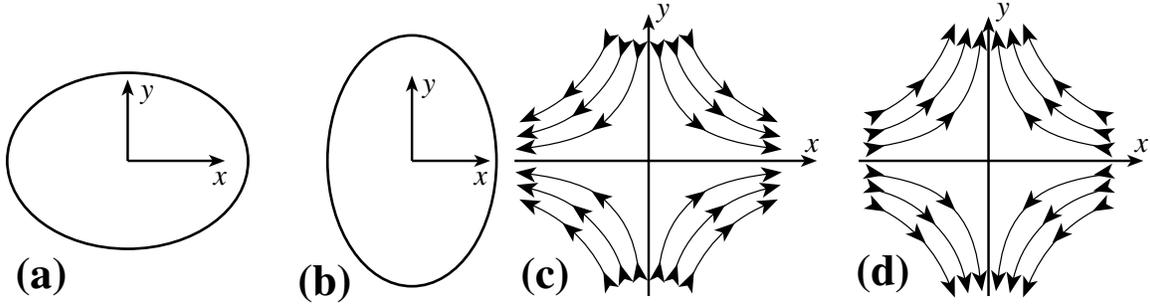
**Fig. 26.1:** Physical manifestations, in a particle's local Lorentz frame, of  $h_+$  gravitational waves. (a) Transverse deformation of an initially spherical cloud of test particles at a phase of the wave when  $h_+ > 0$ . (b) Deformation of the cloud when  $h_+ < 0$ . (c) Field lines representing the acceleration field which produces the cloud's deformation, at a phase when  $\ddot{h}_+ > 0$ . (d) Acceleration field lines when  $\ddot{h}_+ < 0$ .
